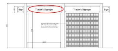
Trader signboards will be fixed to the header boards using studs so they will be slightly proud of the header. The sides of the signboard will be painted black.
